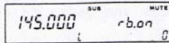
The display shows that both SUB band mute and SUB band beep functions are ON.
